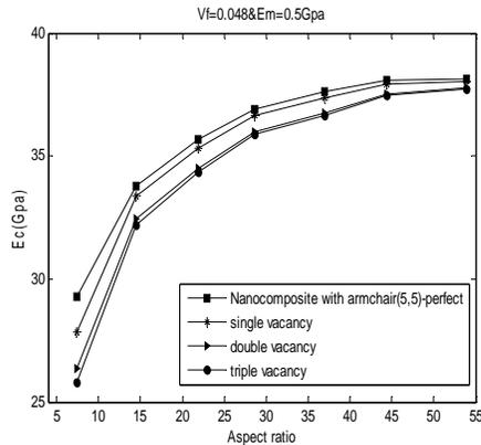
**Fig. 7** Variations Young's modulus RVE for different types defects respect to aspect ratio and compare with armchair(10,10), perfect model nanocomposite, (long CNT inside matrix,  $V_f=0.048$  and  $E_m=0.5$  GPa).
