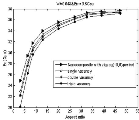
**Fig. 6** Variations Young's modulus RVE for different types defects respect to aspect ratio and compare with zigzag (10,0) perfect model nanocomposite , (long CNT inside matrix,  $V_f=0.048$  and  $E_m=0.5$  GPa).
