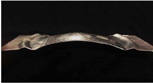
Fig.4 A view of deformed 75 mm×200 mm specimen.
