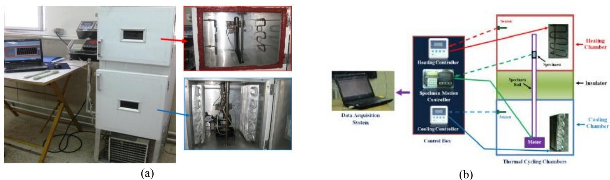
Fig.2 Thermal cycling two chambers apparatus a) picture of the apparatus, b) schematic diagram of the apparatus.
