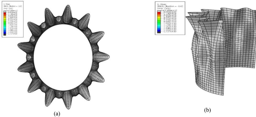
**Fig.2** First buckling mode using Abaqus code ( $\varepsilon / h = 1$  and  $\lambda_{\max} / \lambda_{cl} = 0.893$ ) (a) axial view and (b) lateral view.
