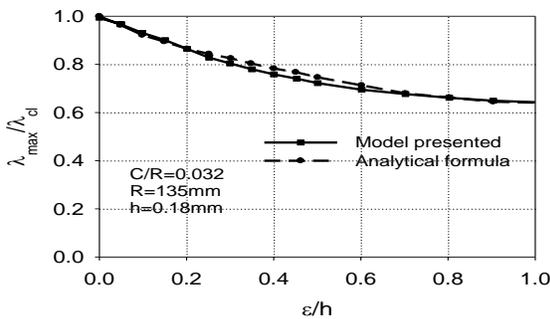
**Fig.4** Evolution of the critical load according to the reduced amplitude  $\varepsilon/h, \zeta = 4.32\text{ mm}, \beta = 2, n = 15$  : Comparison between numerical model and analytical results for the reduction of the critical load.
