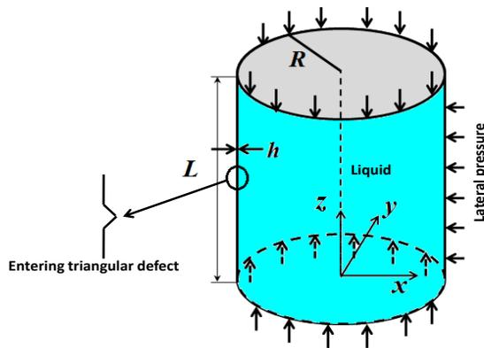
Fig.1 Geometry and coordinate of the axially compressed cylindrical shell.
