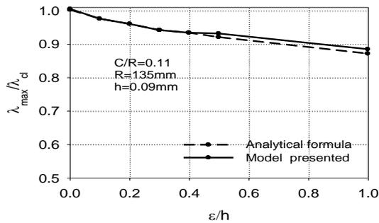
**Fig.3** Effect of the shape defect:  $\varepsilon/h, \zeta = 4.32\text{ mm}, \beta = 2, n = 15$  : Comparison between numerical model and analytical results for the reduction of the critical load.
