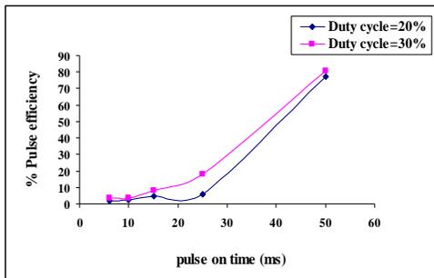
Fig. 4 The influence of the pulse-on time and duty cycle on the pulse efficiency in positive polarity.
