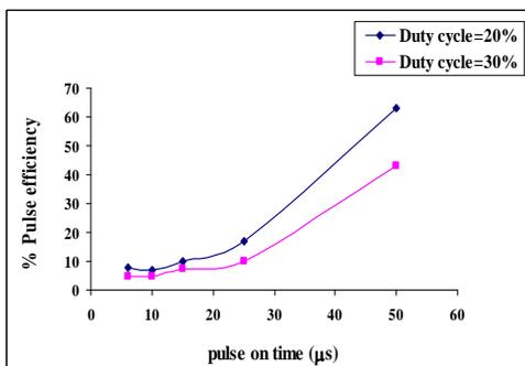
Fig. 5 The influence of the pulse-on time and duty cycle on the pulse efficiency in negative polarity.
