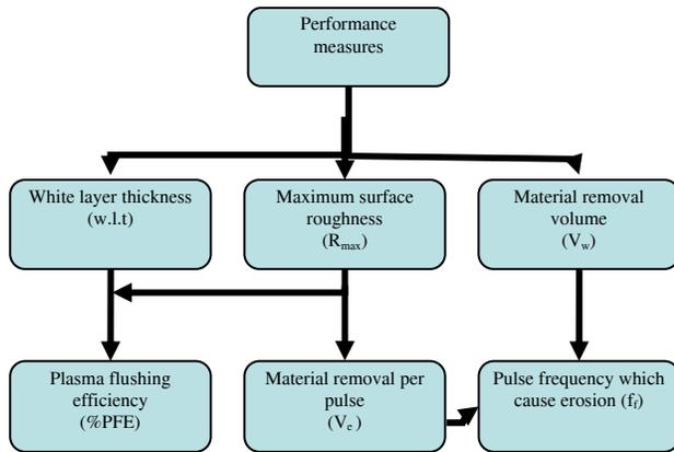
Fig. 3 Process of calculating the pulse efficiency and (%) PFE.
