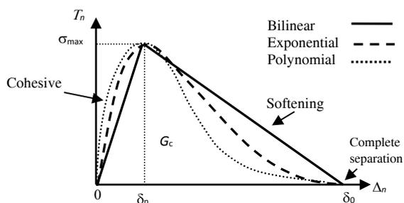
**Fig. 2** Three common categories of traction-separation laws.
