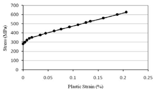
**Fig. 6** Stress- plastic strain curve given for the Multi-linear Isotropic Work Hardening model.
