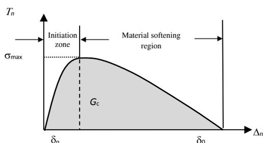
**Fig. 1** Schematic of cohesive model (damage is localized at the interface) and a typical stress-traction variation at the interface.
