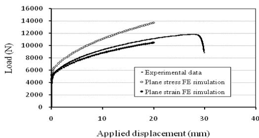
**Fig. 7** Elasto-plastic FE simulation of the tensile test specimen.
