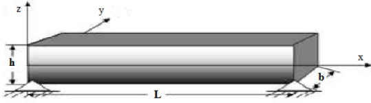
Fig.1 Geometry of FGM beam and the possible variation of ceramic and metal through thickness.
