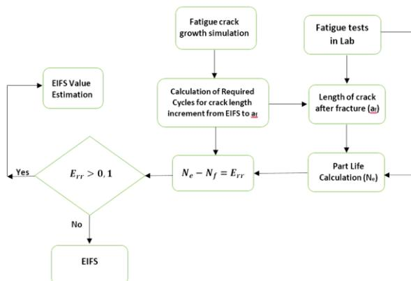
Fig.2 Extrapolation method for EIFS calculation.
