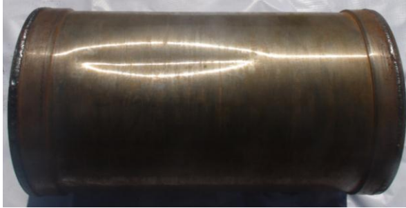
Fig.11 Buckling mode shape after test.
