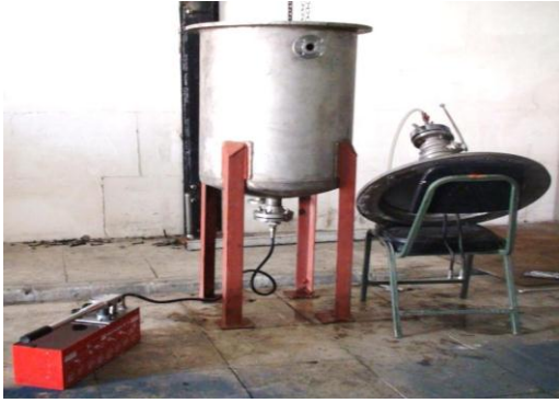
Fig.8 External hydrostatic pressure testing apparatus.
